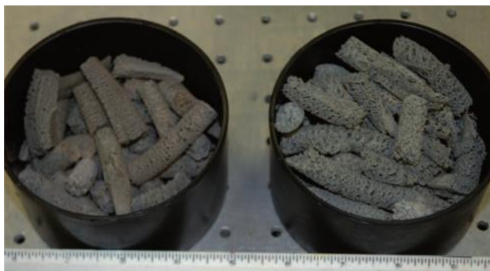
Figure 1.6. Co nanofoams prepared by the combustion of cobalt bistetrazolamine complex with porosity ranging from nm to mm. Adapted with permission from reference 5. Copyright 2010 John Wiley and Sons, Inc.
